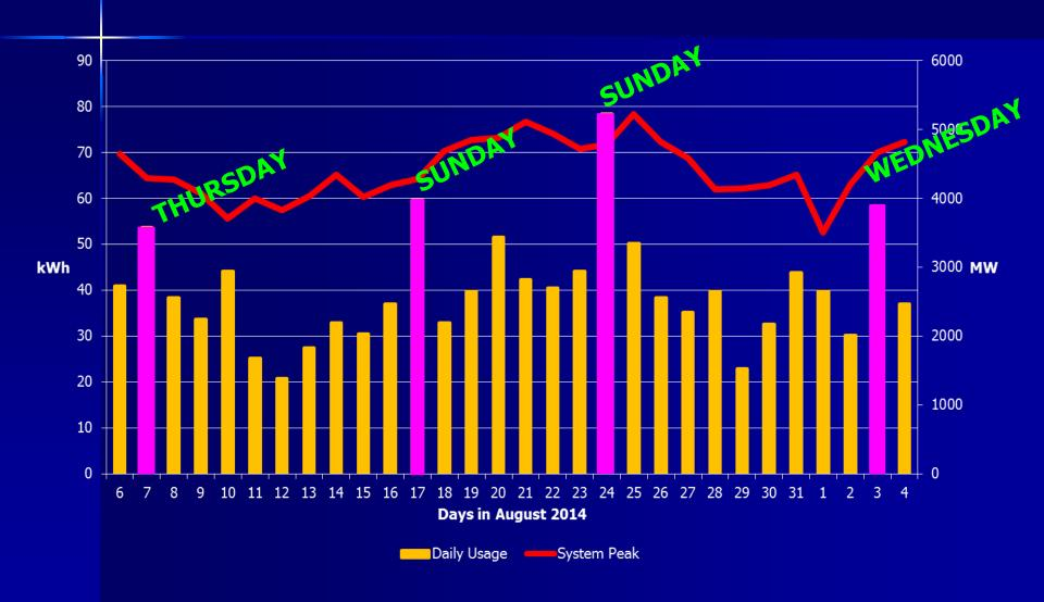
August 7, 2014 kWh usage (15 minute increments) vs Hourly System Load (MW)
