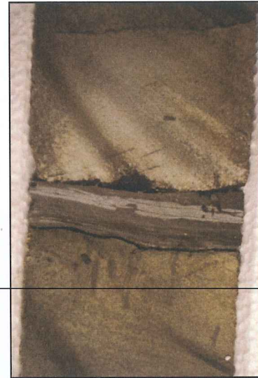
the Saline Aquifer Test Center project in Escatawpa, Mississippi. Note the shale stringer in the sandstone of the lower Tuscaloosa Formation.
