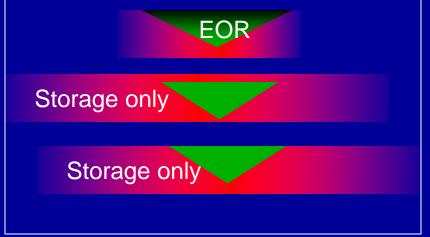
By developing multiple injection zones beneath the EOR zone, the footprint of the CO<sub>2</sub> and pressure plume can be minimized and storage volume maximized
